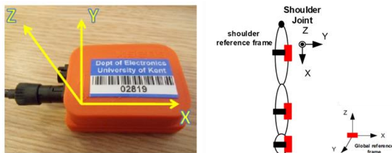
Figure 1 Reference frames for the XSens MTx inertial sensor system.
