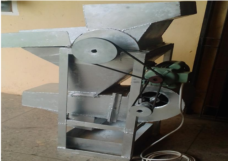
Figure 2 The fabricated cowpea threshing machine
