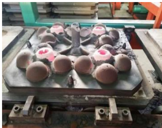
Figure 1 Machine moulding and pairs of grinding media balls
