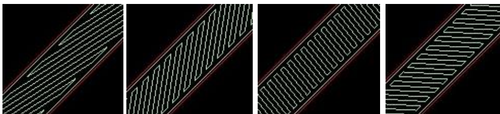
Figure 5 Extruded fibers orientation – sample 3
