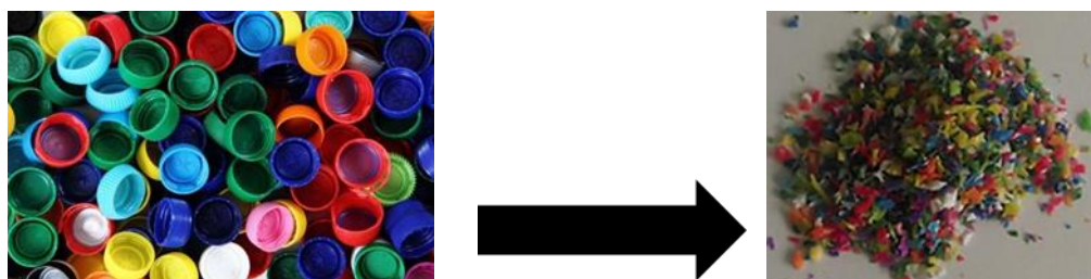
Figure 4 The disintegration of PET bottle lids
