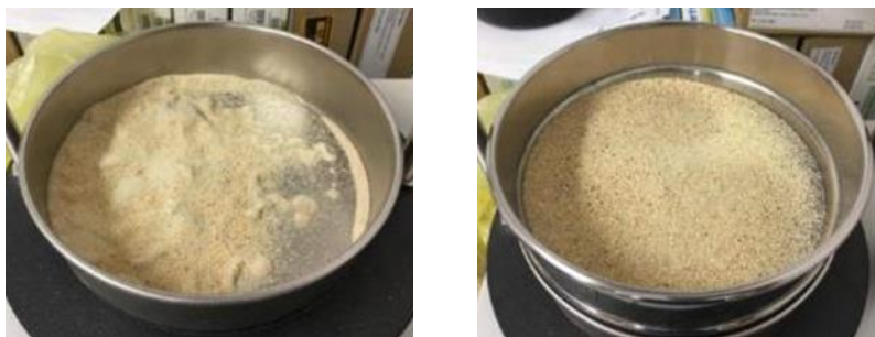
Figure 3 Spruce sawdust in samples suitable for WPCs production – up to 0.5 mm sawdust (left), up to 1.0 mm (right)
