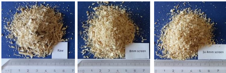
Figure 1 Shredding of spruce chips to the samples of spruce sawdust - raw spruce chips (left), sample after 1st level of shredding (middle), sample after 2nd level of shredding (right)
