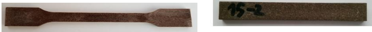
Figure 5 Testing specimens after injection – specimen for tensile test (left), specimen for impact test (right)
