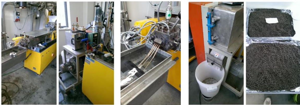
Figure 6 Extrusion and production of composites granules by twin-screw extruder
