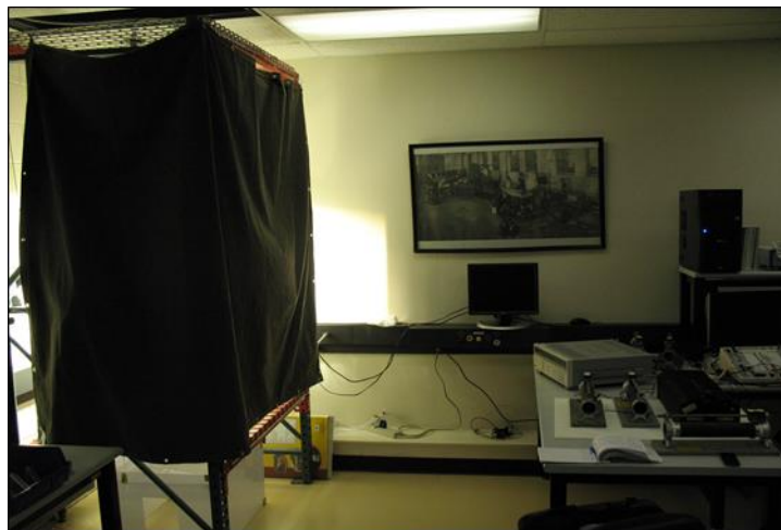
Figure 2c Pictorial view of the solar simulator along with apparatus used load circuit while testing of amorphous silicon panel
