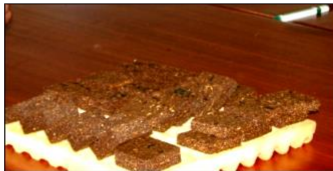
Figure 4 Soaked specimens for dimensional stability test
