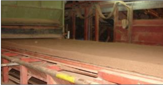
Figure 2 Cold pressed mat formed from blended particles
