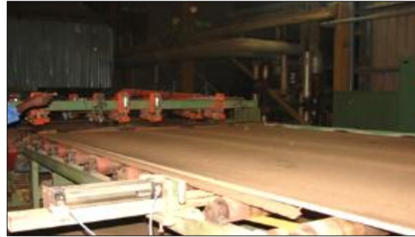
Figure 3 Pressed panel being edge-trimmed
