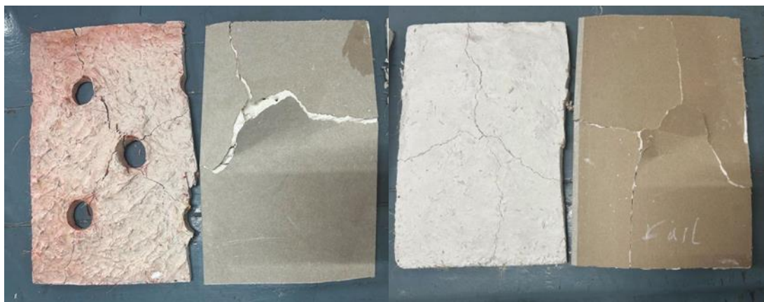
Figure 5 Impact strength test result of cast vs conventional panel.
