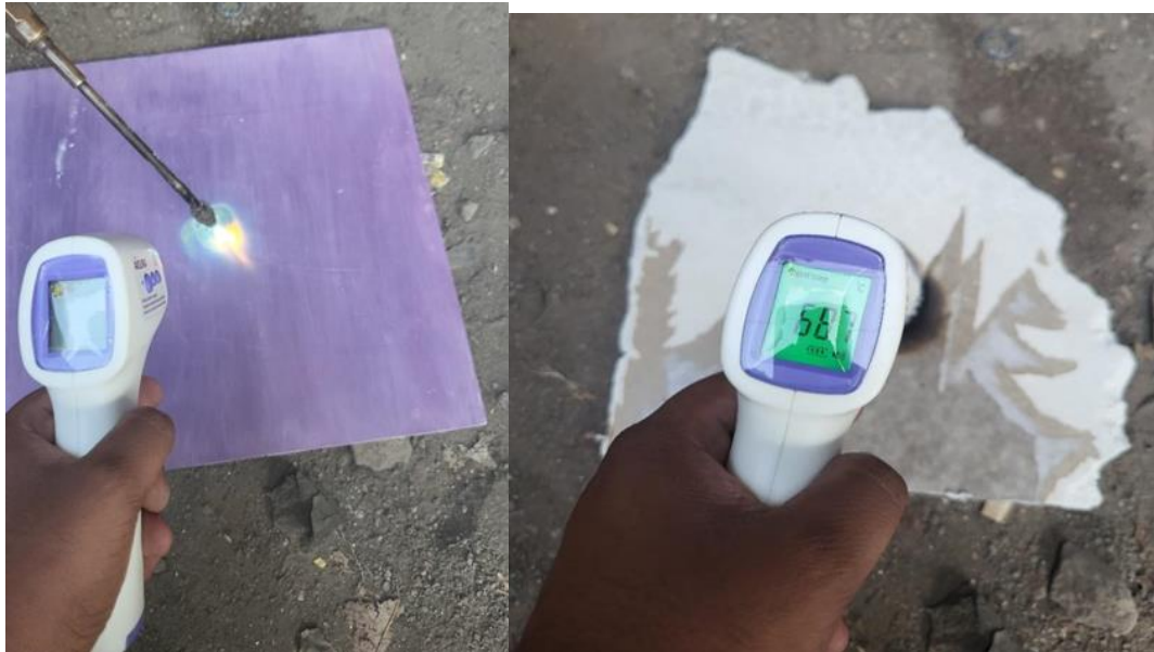
Figure 4 Test setup of thermal resistance test.
