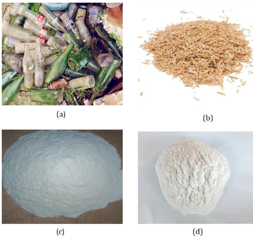
Figure 1 Representative pictures of (a) waste SLSG (b) RH (c) recycled SLSG (d) RHA
