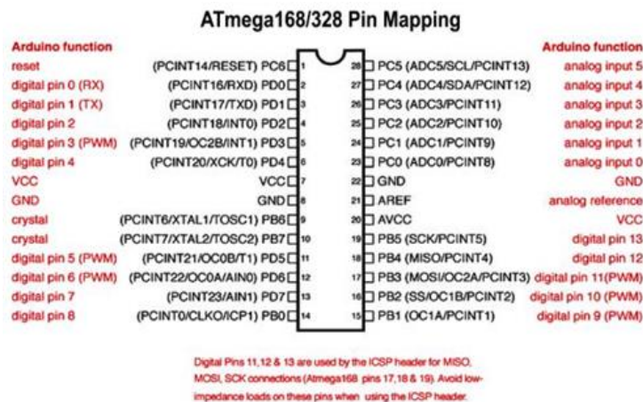
Figure 7 Atmega168/328 IC Architecture Layout
