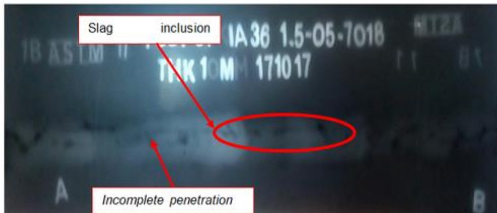
Figure 7 The results of underwater welding radiography with electrodes E7018 at a depth of 5 meters and heat input (HI) 1.5 kJ/mm
