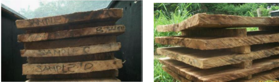
Figure 1 Wood stacked in the solar kiln and wood stacked in open air environment
