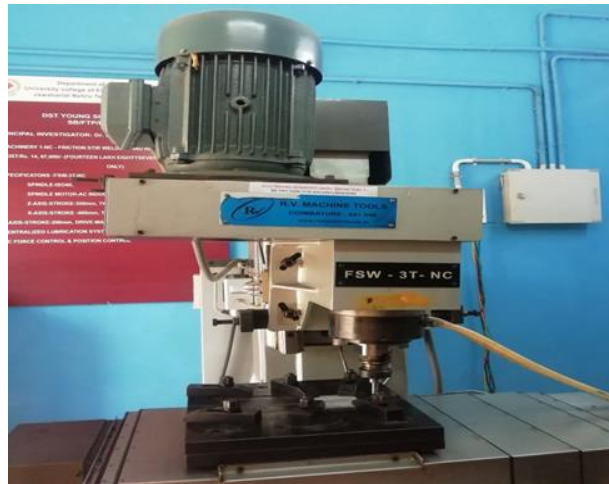
Figure 1 Friction Stir welding Setup
