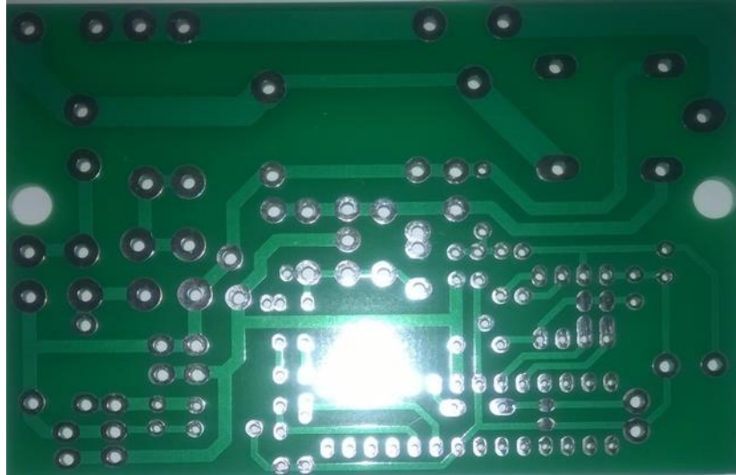
Figure 7 The printed circuit board is designed to integrate the voltage converter block, light sensor, real time and automatic load shedding power block
