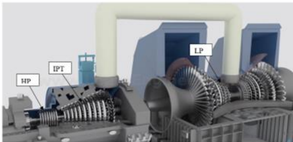
Figure 2 Turbines section of the power plant
