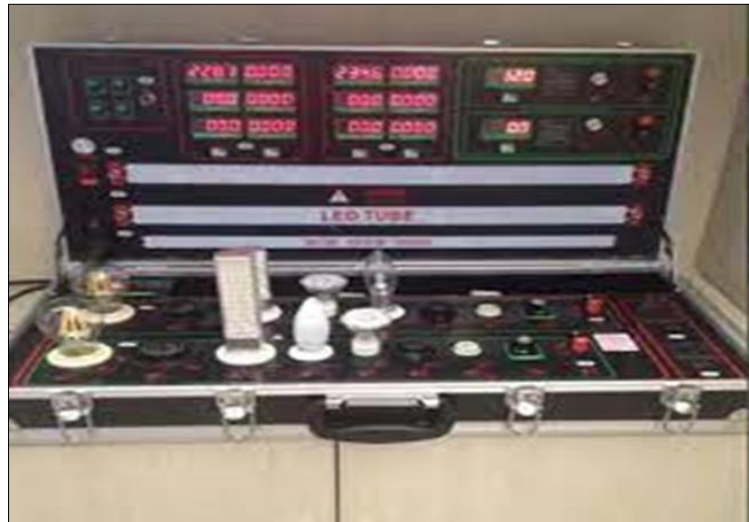
Figure 2 New double T8 full range & ac/dc power meter with dimmer
