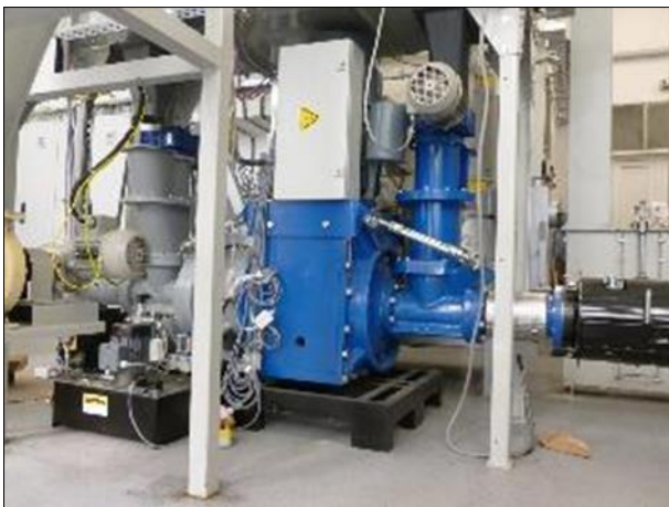
Figure 9 Developed two-chamber screw press located in the technological briquetting line
