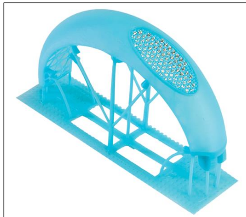
Figure 7 Model made of Wax Castable Resin material [18]
