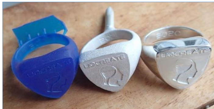
Figure 6 Liqcreate wax castable casting process [17]
