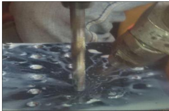
Figure 2 Application of Neem oil on the drilling zone
