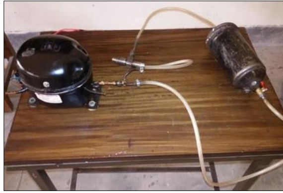
Figure 1 MQL system set-up
