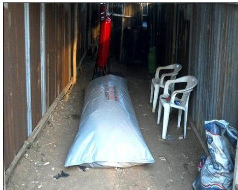
Figure 2b Gas storage bag filled with pyrolysis gas (after experiment)
