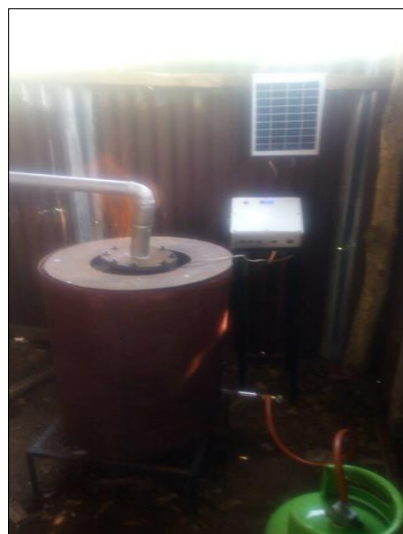
Figure 3 Gas-fired furnace with attached solar-powered temperature sensor
