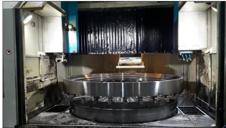
Figure 1 Vertical lathe machining a bearing ring
