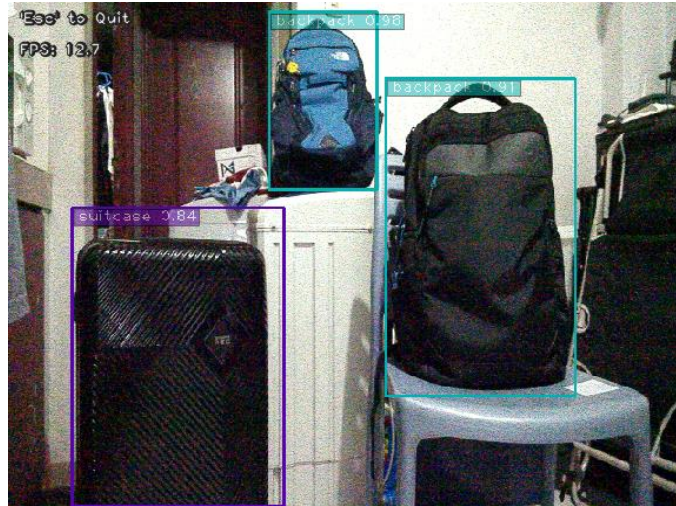
Figure 6 Sample detection on Jetson TX2 development kit using SSD
