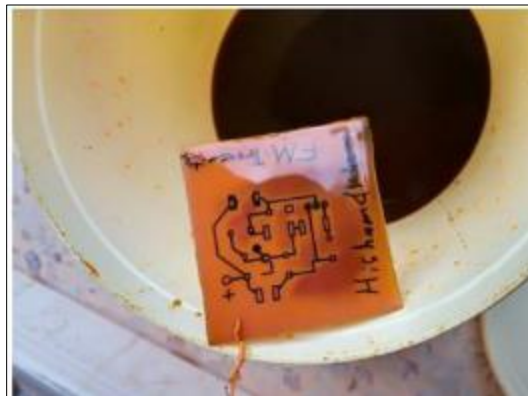
Figure 23 Remove the Copper with \text{FeCl}_3
