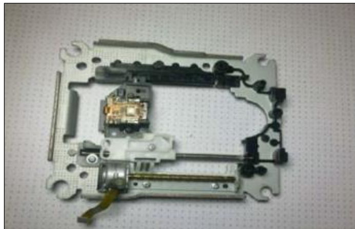
Figure 6 DVD driver servomechanism
