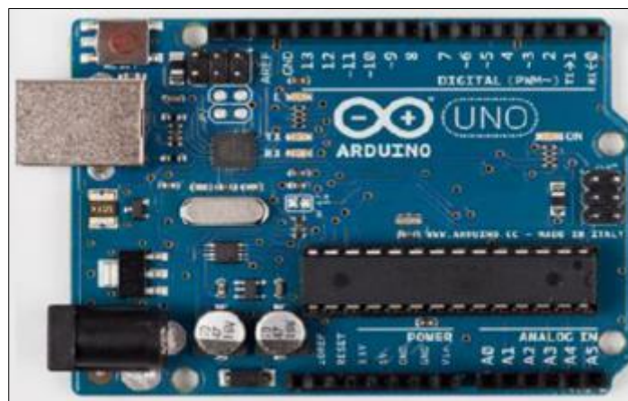
Figure 9 The Arduino UNO board
