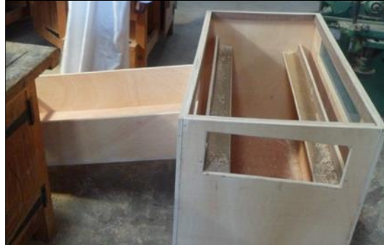
Figure 2 Inner view of the solar dryer
