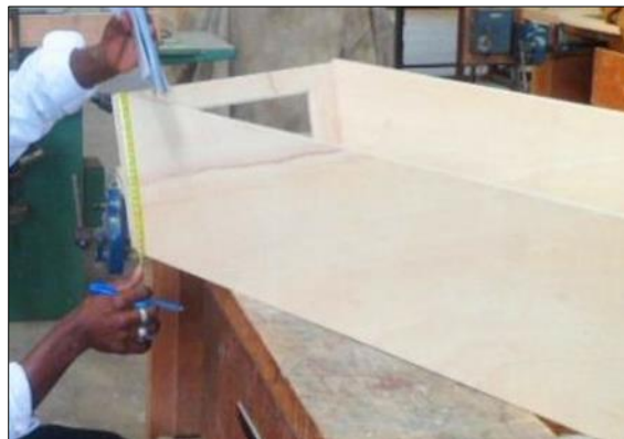
Figure 3 Constructed solar collector
