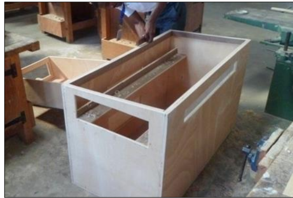
Figure 4 Coupling the collector & drying chamber
