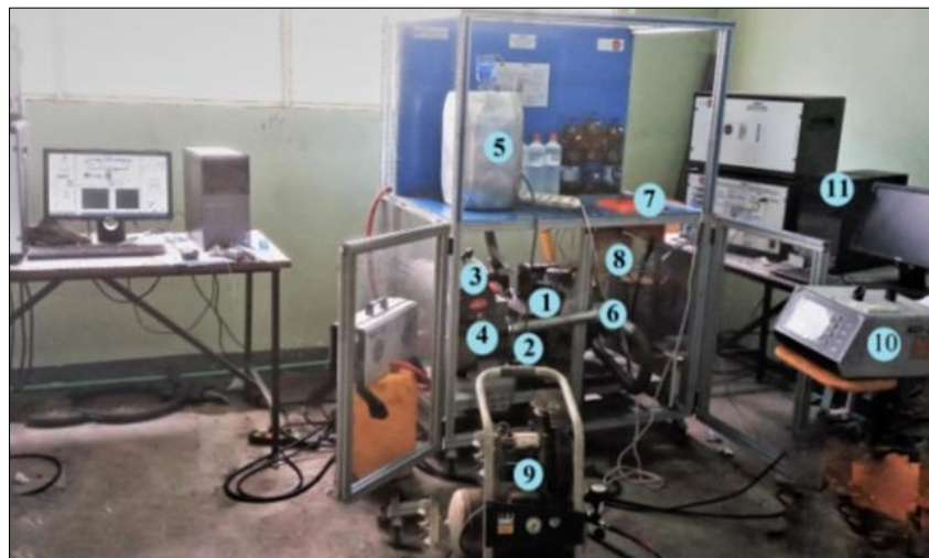
1-Engine, 2-Motor, 3- EGR cooler, 4- EGR valve, 5- Coolant reservoir, 6-Intake port, 7- Diesel reservoir, 8- Methanol reservoir, 9- Air Compressor, 10- Smoke meter, 11- Control unit.
