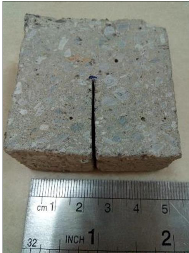
Figure 7 water flow sample with artificial concrete crack
