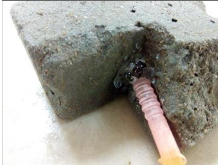
Figure 11 A UHAP capsule cracked open inside the concrete mass, ejected sealing gel
