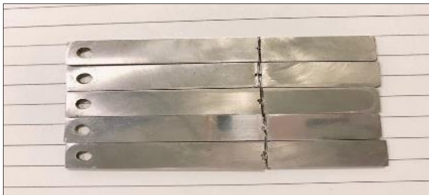
Figure 14 The location of the fracture in the samples (CH)
