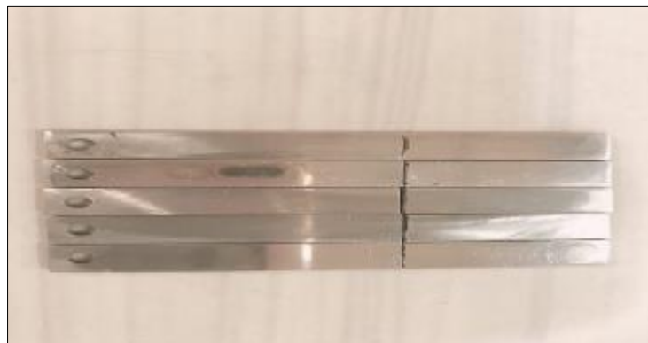
Figure 12 The location of the fracture in (BM)
