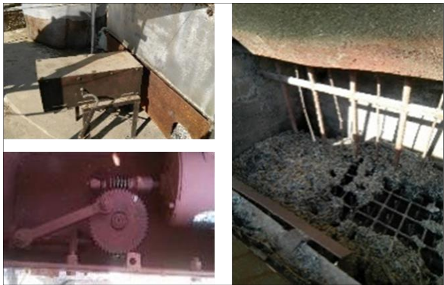
Figure 3a Grate shaker with worm gear and slider crank arrangement and comber
