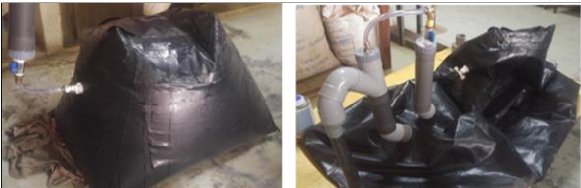
Figure 4 (Left) Water Tight test on Gas Storage. (Right): Mounted system after various test
