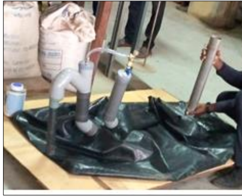
Figure 3 Complete 300L prototype biodigester ready for feeding
