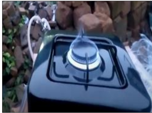
Figure 17 Burning biogas from prototype digester
