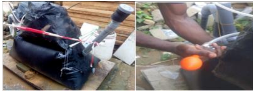
Figure 7 (Left): Prototype biodigester after HRT; (Right): Gas sample collection
