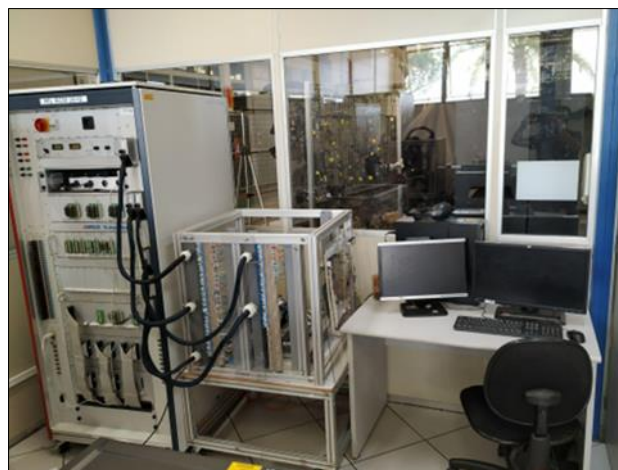
Figure 13 ECU and Simulator Connection in Platform.
