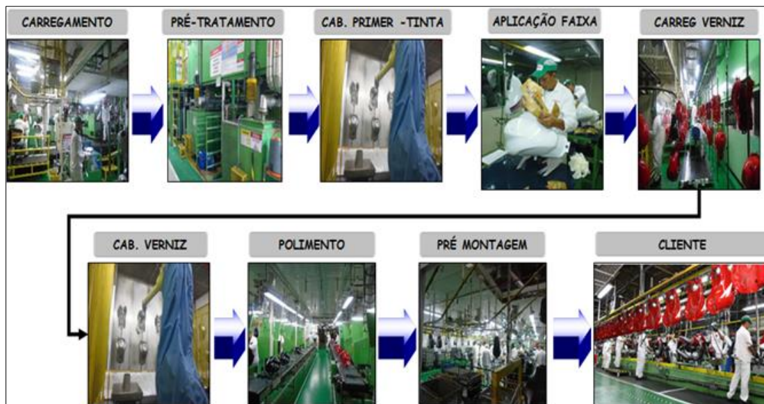
Figure 2 Flow of the metallic parts process
