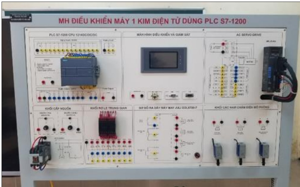
Figure 6 JUKI DDL 8700-7 single-needle machine control model using PLC S7-1200
