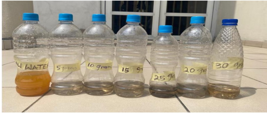
Figure 5 Treated effluent sample from varying adsorbent dosage.
