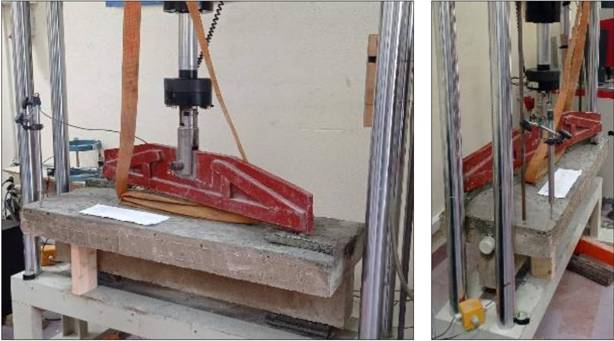
Figure 3 Test configuration, loading position and position of LVDT and torsion angle metering system
