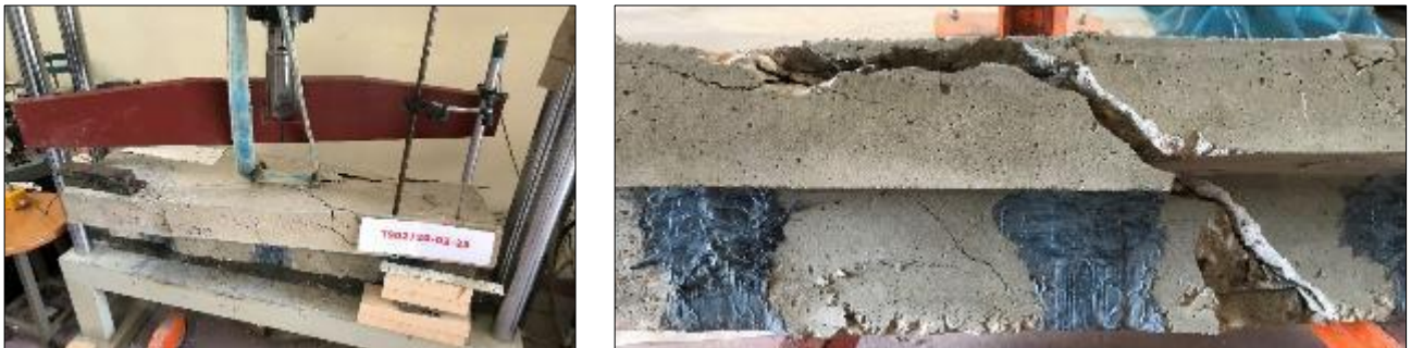
Figure 6 Crack pattern of the sides of the U-jacketed FRP strips at strengthened beam TS02
