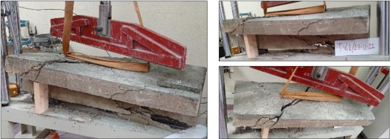
Figure 4 Crack pattern of control beams TV01
