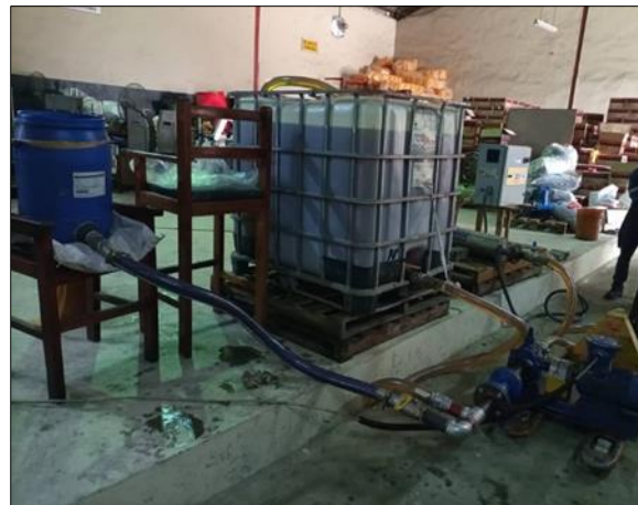
Figure 3 Ultrasonic processor method with introduction of separate additive container
