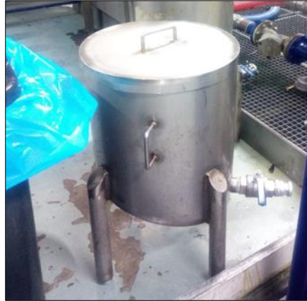
Figure 6 Additives Preheating Tank for SAE 30 marine oil
