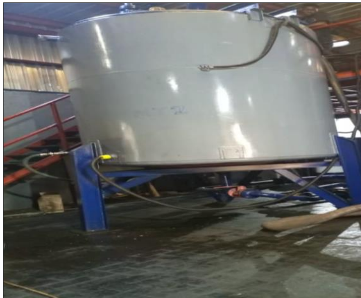
Figure 8 Blending kettle used for Marine Grade SAE 30 Lubricant
