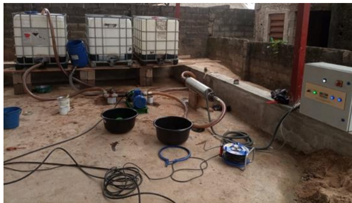
Figure 7 Marine grade SAE 30 blending using ultrasonic processor
