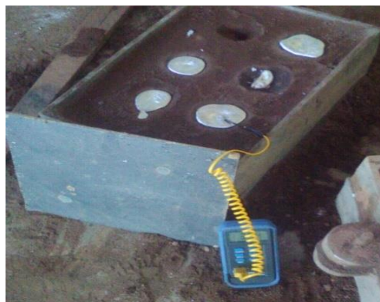
Figure 2 The solidification process of the casted specimens
