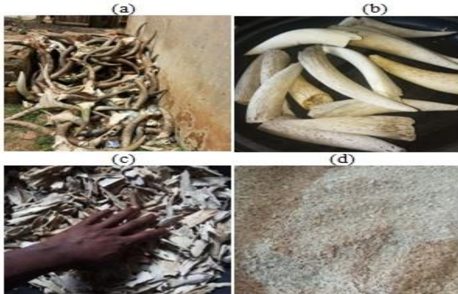
Figure 1 (a) Raw cow horns (b) Thoroughly washed and sun-dried cow horns (c) Crushed cow horns (d) grinded cow horns (cow horn particulates)
