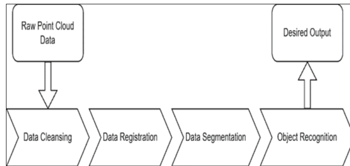
Figure 4 Typical Processing Procedures of Point Clouds Data
