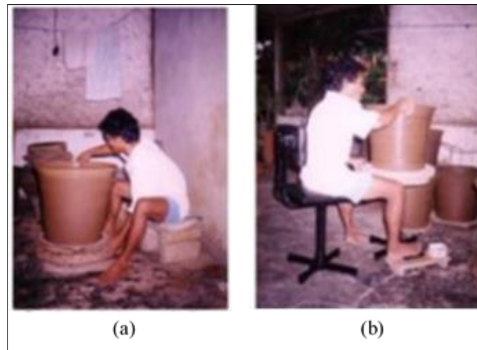
Figure 5 Redesign of pottery-making work tools a) old tools, b) redesigned tools [20]
