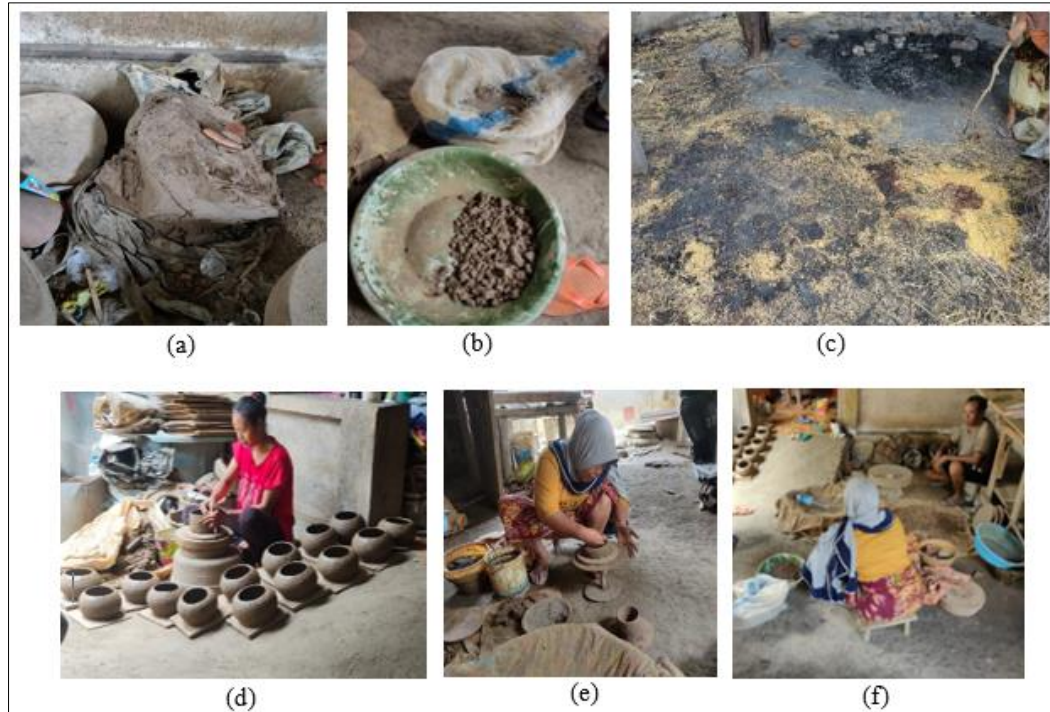
Figure 1 Simple tools and working postures in making pottery, a) clay, b) tools for mixing clay, c) firing pottery and d), e), f) forming process [4]
