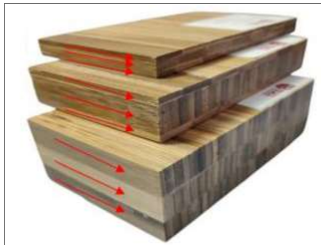
Figure 2 Paralel lay up of bamboo strip
