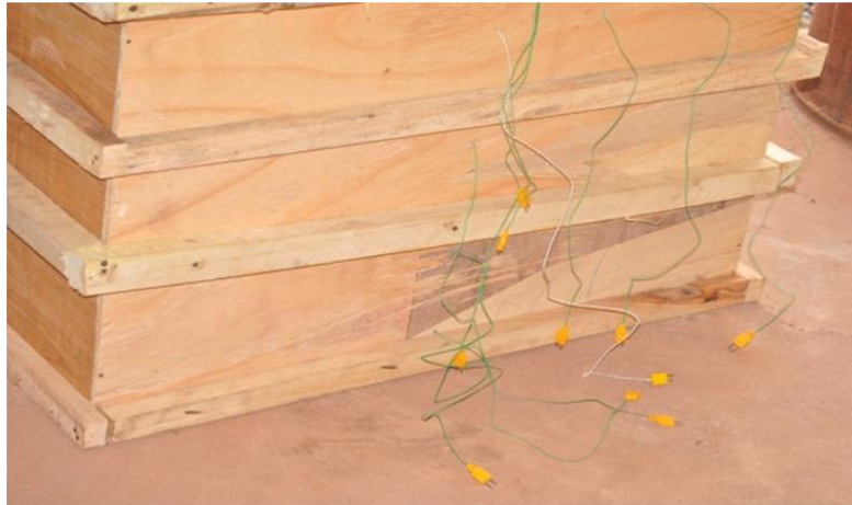
Figure 3 Cast concrete block with the thermocouples (mix 1:2:4).
