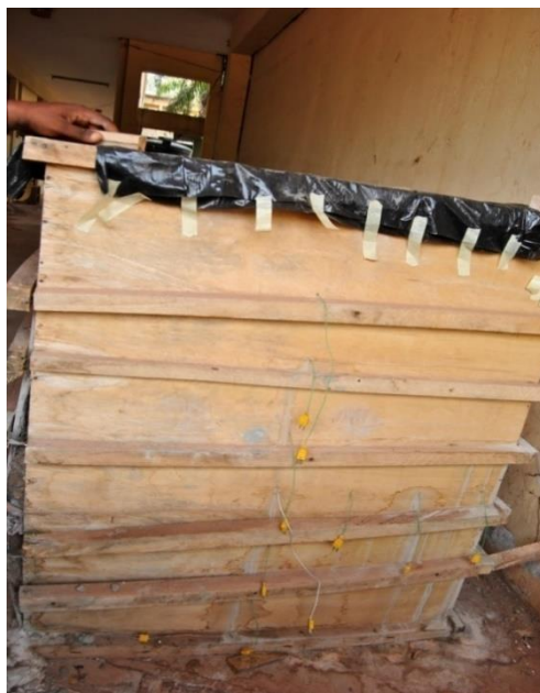
Figure 4 Cast concrete block with the thermocouples (mix 1:3:6).
