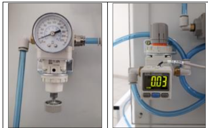
Figure 5 AR-B Series Modular Pressure Regulator - AR20-01BG-B and Flow Meter. ISE30A-01-N-LD series high precision digital pressure switch. Source: From the author (2021)
