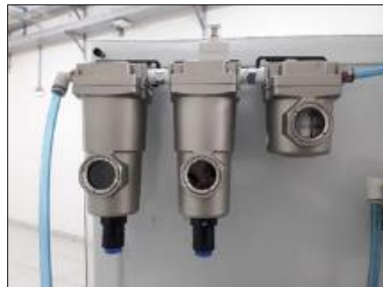
Figure 3 Industrial Filters. Mix of industrial filters containing SMC Condensate Separator Air Filter, model AMG150C-02BD; SMC 2-stage Submicron Air Filter, model AMH150C-02BD-T. Source: From the author (2021)
