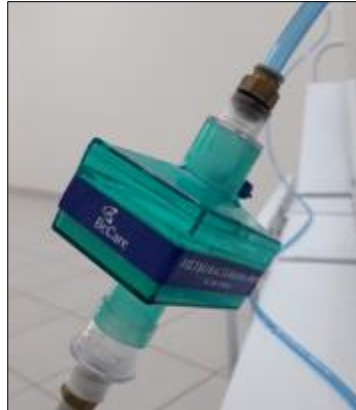
Figure 4 HEPA filter. BECARE brand hospital standard HEPA bacterial filter, dimensions 5x10x7 cm. Source: From the author (2021)
