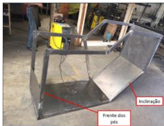
Figure 7 Initial construction: metal bars and metal sheets. Source: From the author (2021)
