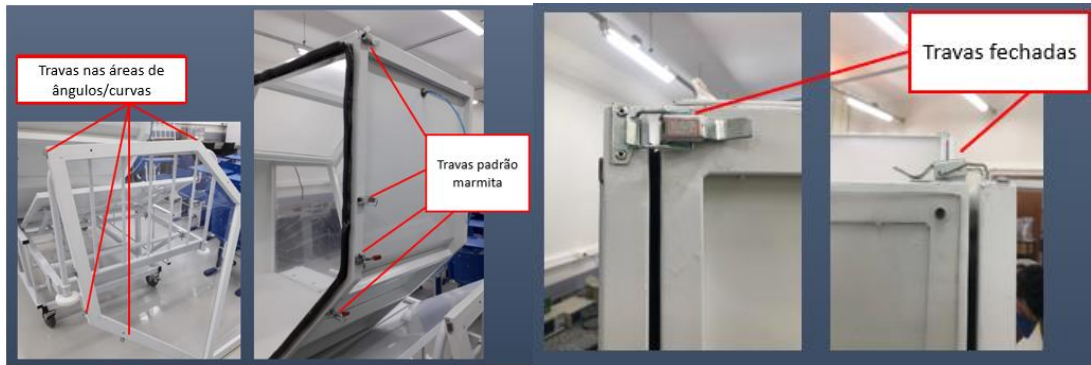
Figure 10 View of the acrylic and rubber sealing plates. Door view of the innovative insulation and transport system. Source: From the author (2021)
