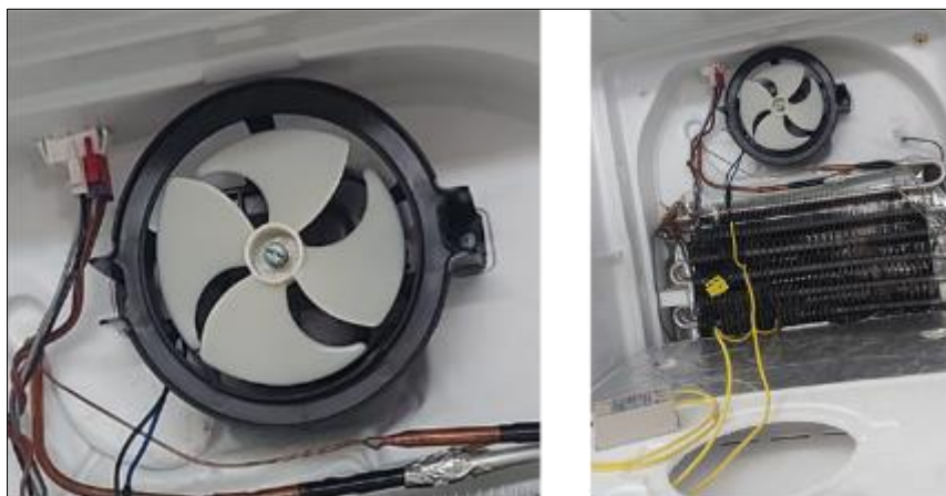
Figure 2 Refrigerator fan A and fault simulation
