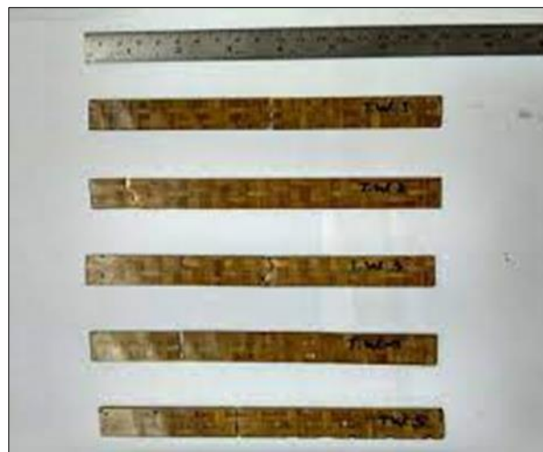
Figure 2 The polyester composites with reinforced Bambusa maculata fibers
