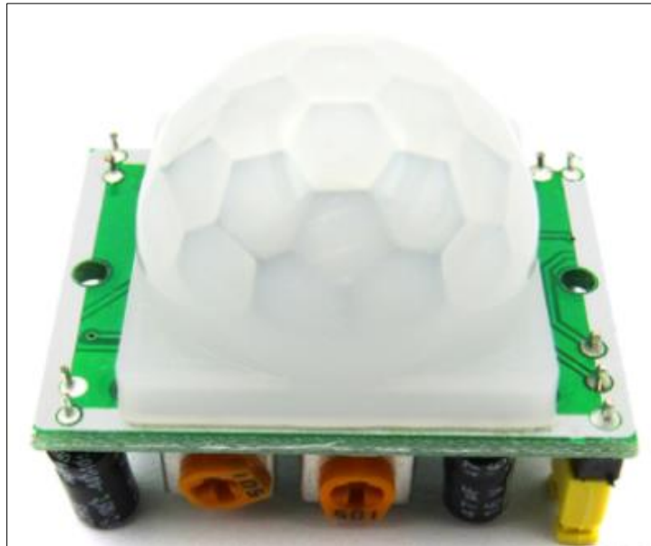
Figure 3 The HC-SR501 human infrared sensor
