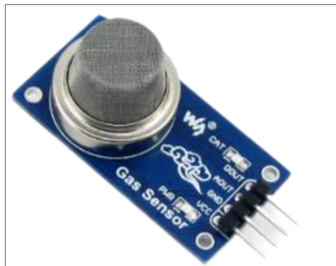
Figure 2 MQ-5 gas sensor
