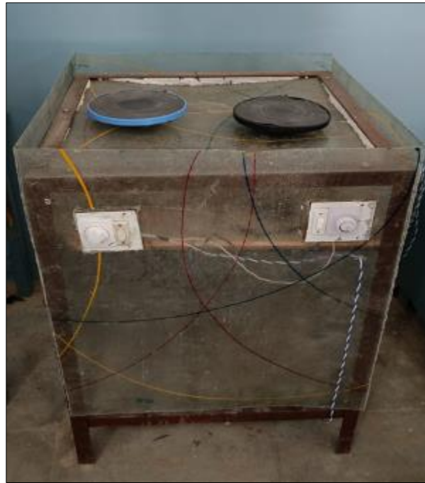
Figure 7 Experimental Setup of double disc polishing machine
