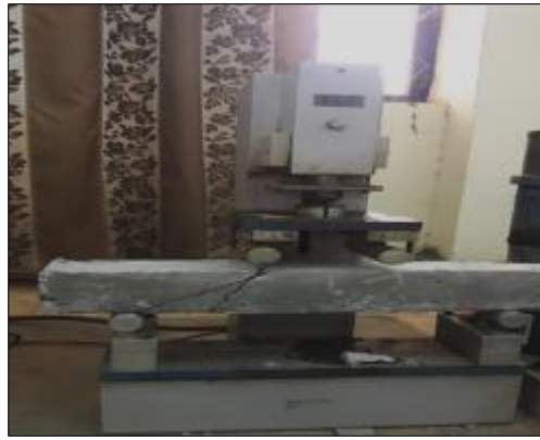
Figure 1 Failure Mode of Reference Beam
