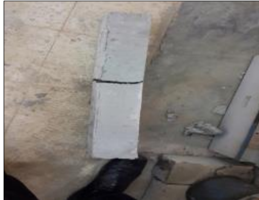
Figure 3 Failure Mode of Bamboo Reinforced Beam
