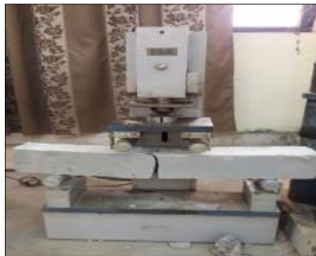
Figure 2 Failure Mode of Palm Leaves-Reinforced Beam
