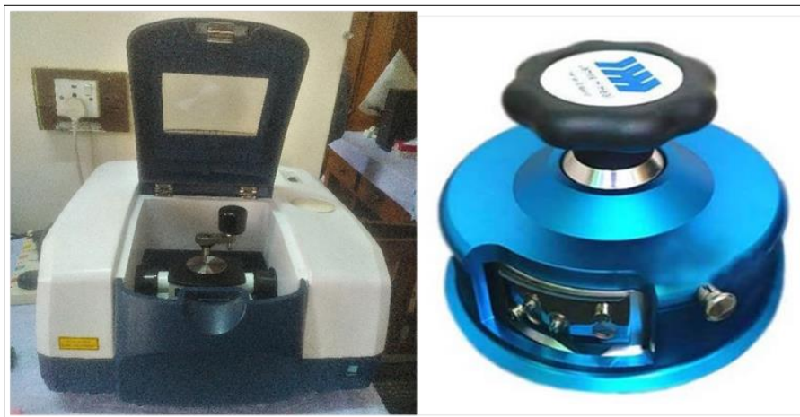
Figure 3 a) FTIR spectroscopy tester b) GSM cutter (James heal)
