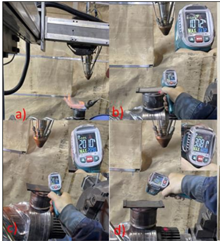
Figure 3 (a) preparation for heating; (b) heating at 100 °C; (c) heating at 200 °C; (d) heating at 300 °C
