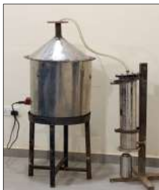
Figure 1 Essential oil extractor
