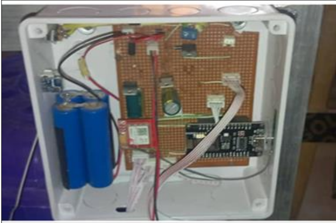
Figure 2a Internal features of the transmitting unit
